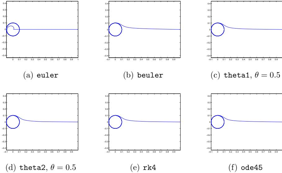
Figure 3: Computation of the limit cycle test problem (5.10), with  $u(0) = (1, 0)$ , using different numerical methods. For each method,  $t \in [0, 100]$  and  $\Delta t = 0.01$  (except `ode45` is evaluated at 0.01 intervals).
