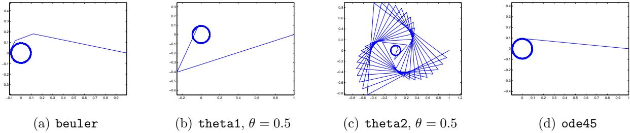
Figure 5: Computation of the limit cycle test problem (5.10), with  $u(0) = (1, 0)$ , using different numerical methods. For each method,  $t \in [0, 100]$  and  $\Delta t = 1$  (except `ode45` is evaluated at 0.1 intervals).
