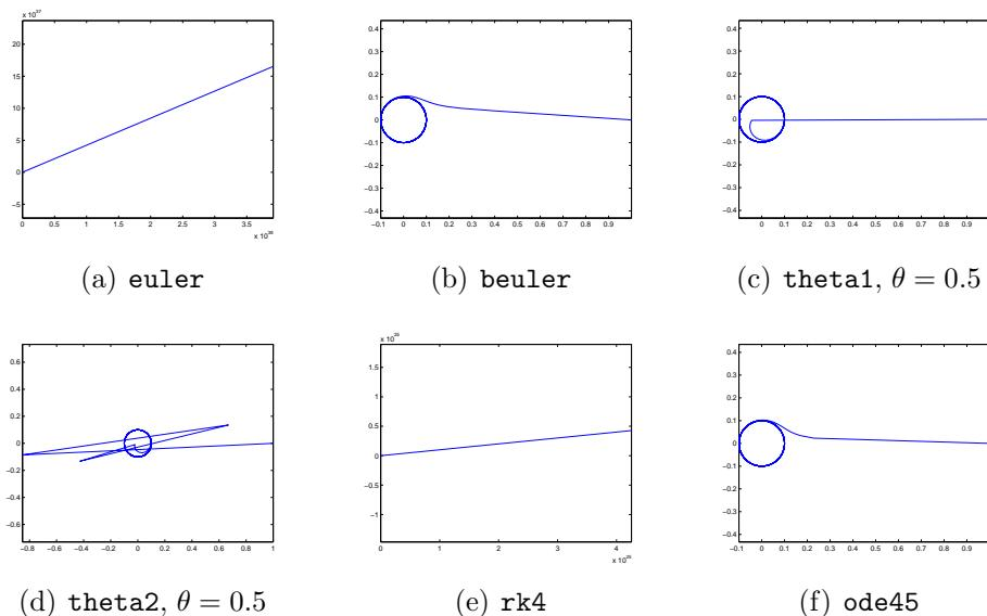
Figure 4: Computation of the limit cycle test problem (5.10), with  $u(0) = (1, 0)$ , using different numerical methods. For each method,  $t \in [0, 100]$  and  $\Delta t = 0.1$  (except `ode45` is evaluated at 0.1 intervals and for `euler`  $t \in [0, 0.4]$ ).
