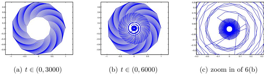
Figure 6: Computation of the limit cycle test problem (5.10), with  $u(0) = (1, 0)$ , using the trapezoidal rule (`theta2`,  $\theta = 0.5$ ) with  $\Delta t = 10$ .
