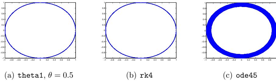
Figure 2: Computation of the simple harmonic oscillator, with  $u(0) = (1, 0)$ , using different numerical methods. For each of the simulations  $t \in [0, 5000]$  and for the first two methods  $\Delta t = 0.1$ .
